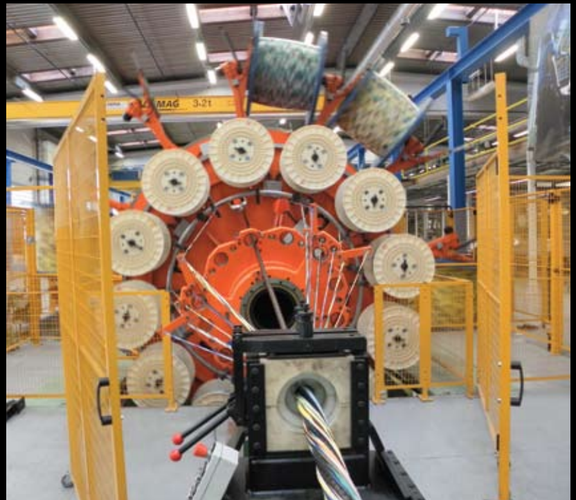
EMEC cabling assembly through the Draka factory. The picture shows the laying up operation of three power cores with additional fillers to circularise the cable. Image by permission of Draka 2010.
