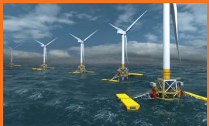
The potential deployment of Wave Treader designed to increase the output of an offshore wind farm.
