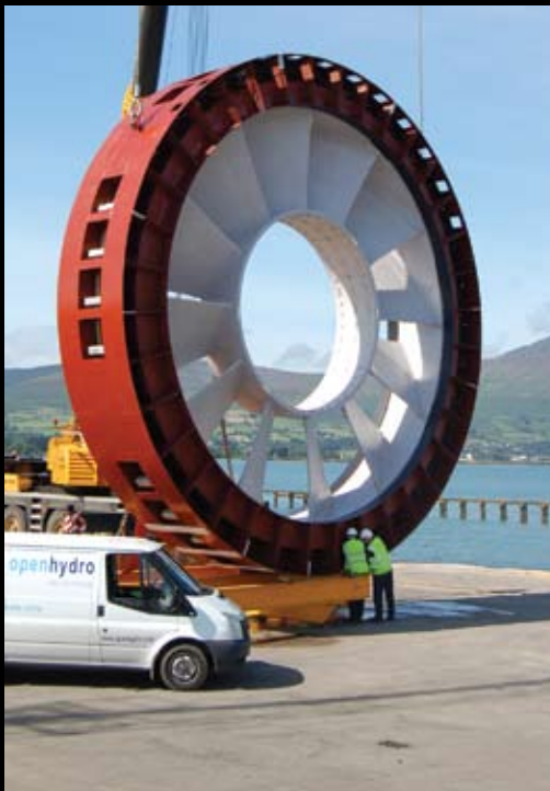
Open Hydro's open-centre 10m turbine that was installed in the Bay of Fundy, Canada, and successive generations of its device continue to be trialled at EMEC.
